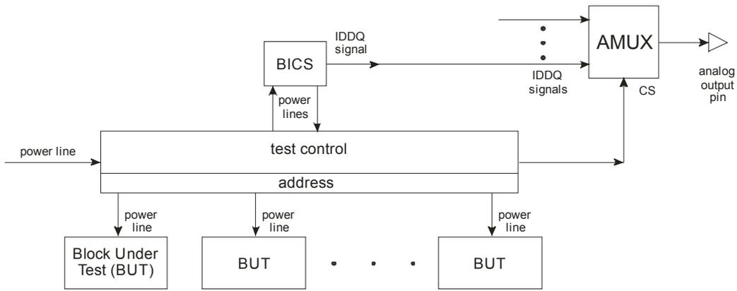
Fig. 1. DFT that enables IDDQ scanning.
