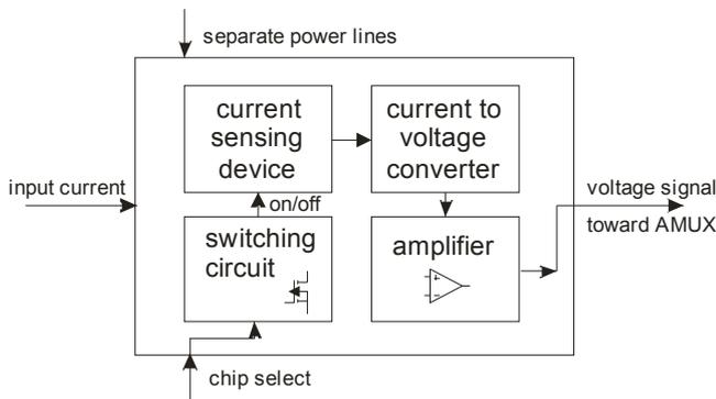
Fig. 2. BICS internal structure.
